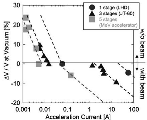
Figure 2. Voltage degradation characteristics depending on acceleration current.  $V$  denotes the acceleration voltage.
