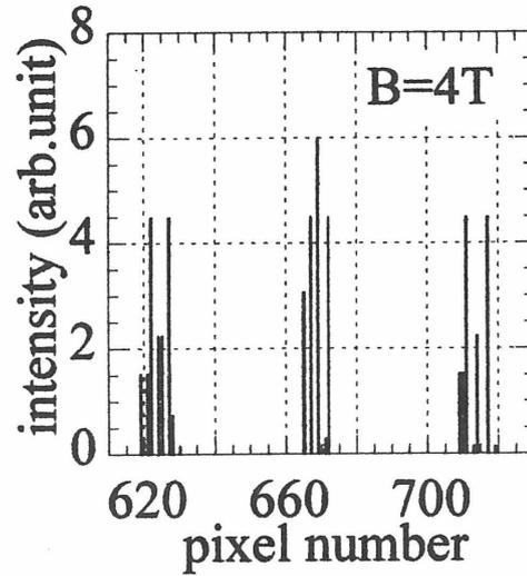
Fig.2. Spectral components of  $H\alpha$  line at  $B=4T$
