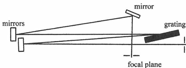
Fig. 1. Optical layout of the high resolution spectrometer with an echelle grating
