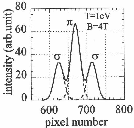
Fig.3. Spectral profile of  $H\alpha$  at  $B=4T$  and  $T_{\text{hydrogen}}=1\text{eV}$
