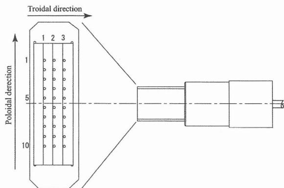
Figure 1. The schematic drawing of 2-D imaging fiber array. This optics enables to obtain poloidal and toroidal distributions of H $\alpha$  emission in same discharge.
