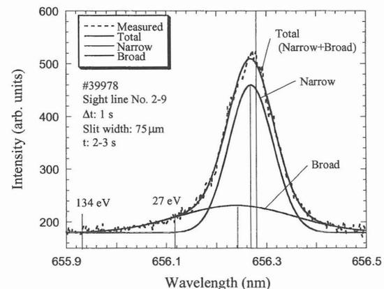
Figure 3. The asymmetric profile of H $\alpha$ . The profile is fitted to a sum of two Gaussian components, narrow and broad. The shoulder in the blue wing is clearly distinguished.
