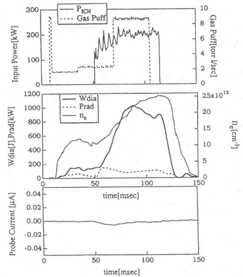
Fig.2 Time evolutions of gas puffing rate, input RF power, stored energy, radiated power, average electron density and helically trapped ion loss with gas puffing during ICRF heating pulse.
