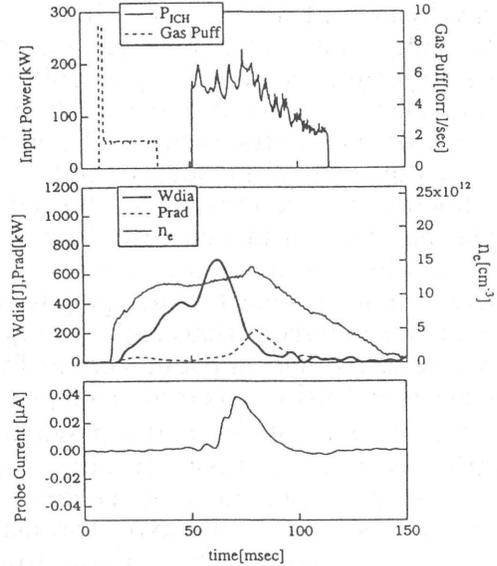
Fig.1 Time evolutions of gas puffing rate, input RF power, stored energy, radiated power, average electron density and helically trapped ion loss without gas puffing during ICRF heating pulse.
