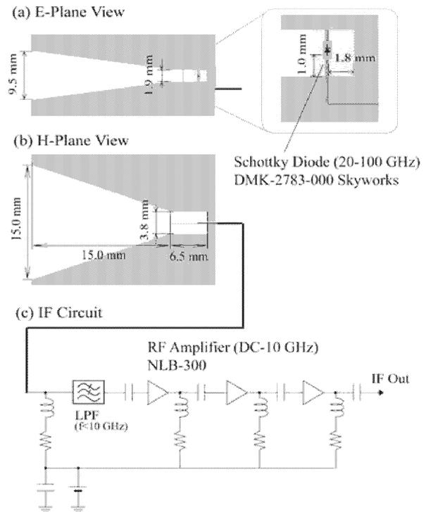
Fig.2 (a) E-plane view and (b) H-plane view of horn antenna element of the V-band (50 to 75 GHz) 2-D antenna array. (c) Schematic diagram of intermediate frequency (IF) circuit on the antenna PCB.
