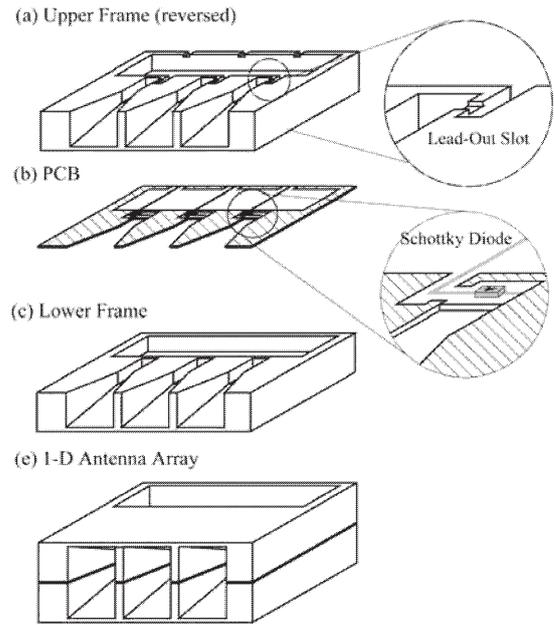
Fig.1 Schematic view of the 1-D horn antenna array assembly. (a) reversed view of upper structure, (b) PCB, (c) lower structure, (d) completed form.
