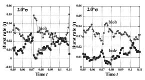
Fig.2 Time evolution of burst rates of blob/hole in the NBI heated Helitron J plasma with SMBI at t=0.072 s for different loaction of the Langumir probe at -4mm inside the LCFS(left), on the LCFS (right).
