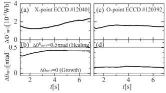
Fig.2 Time evolution of (a, c) plasma response field with m/n=2/1 mode and (b, d) phase difference between RMP and plasma response field. (Left) X-point ECCD. (Right) O-point ECCD
