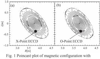
m/n=2/1 magnetic island. Black dot indicates the position of ECCD at (a) X-point and (b) O-point.
