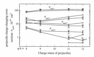
Fig. 1  $\sigma_{q,q-k}$  as a function of projectile charge states q, Solid and open symbols represent experimental results and calculations from classical models.
