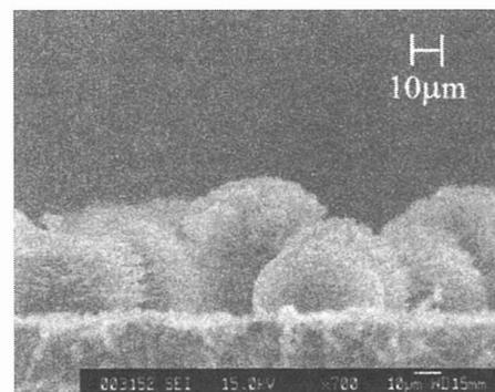
Fig.3 A SEM image of particulates produced on the surface of the carbon target.
