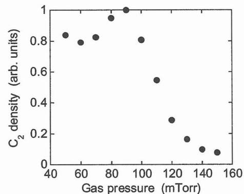
Fig.2 The  $\text{C}_2$  radical density measured by LIF as a function of the gas pressure.
