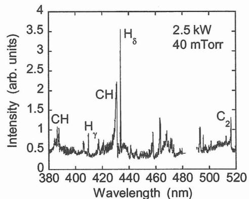
Fig.1 Optical emission spectrum observed from the interface region between the high-density hydrogen plasma and the target graphite plate.
