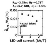
Fig.2(b). Dependence of magnetic fluctuation level on LID current at Bt=0.75T.
