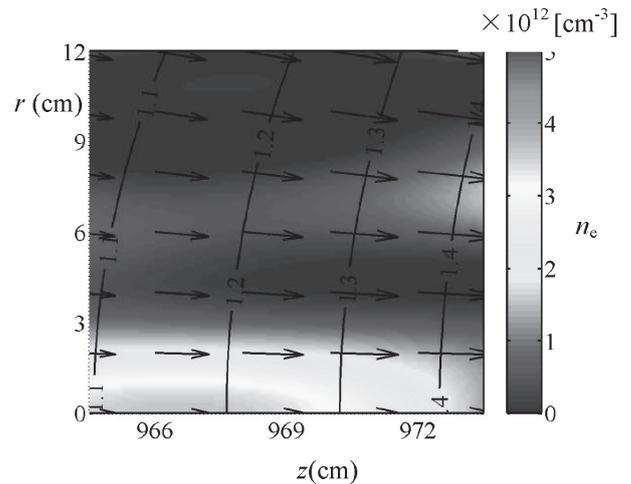
Fig.2. 2D view of the density profile during the ECRH for potential formation is applied.
