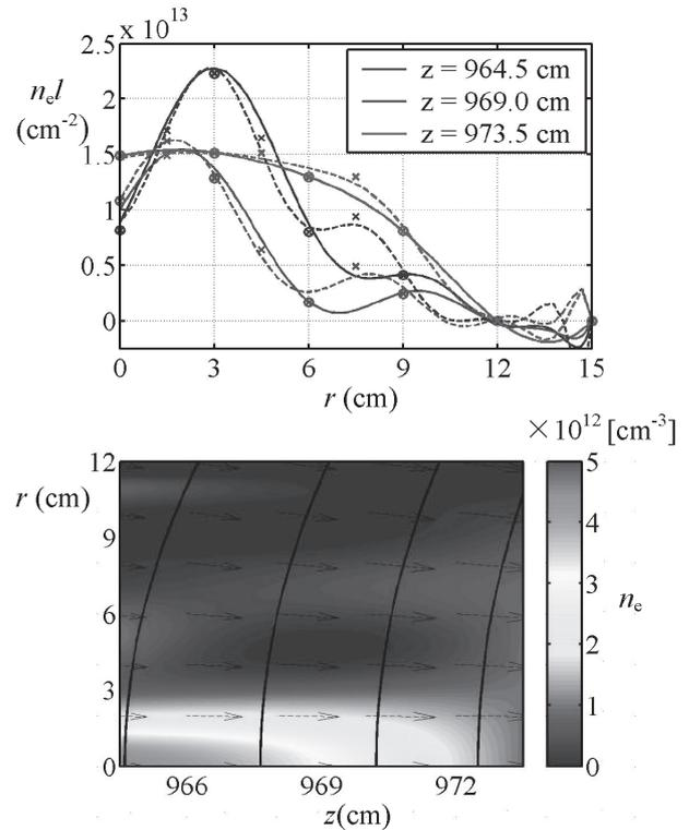
Fig.1. Radial profiles of the line density for various axial positions (top), and 2D view of the Abel-inverted density profile (bottom).
