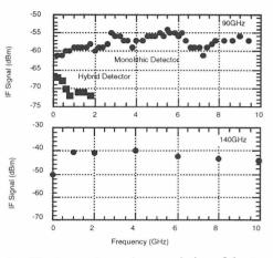
Fig. 1 The heterodyne characteristics of the two-types of detectors.
