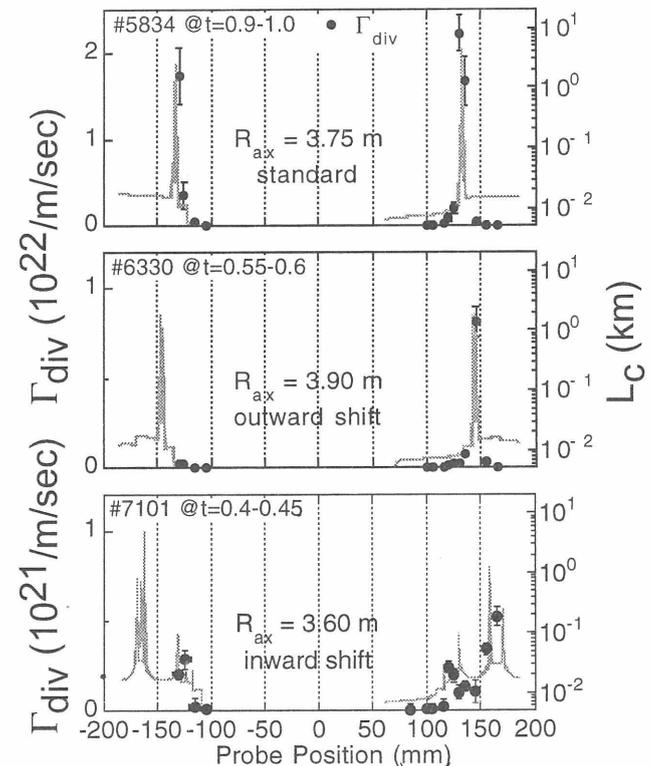
Fig. 1: The profiles of the divertor particle flux on the divertor plate at inboard side for various  $R_{ax}$ .
