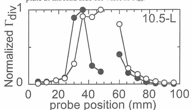
Fig. 2: Normalized divertor particle flux to the divertor plate near 10.5-L port. Closed circles: #11708 ( $\langle\beta\rangle < 1\%$ ) Open circles: #15042 ( $\langle\beta\rangle > 2\%$ )
