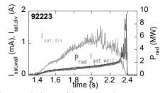
Fig. 3 Time evolutions of ion saturation current to a divertor plate and first-wall, respectively, and radiation power during a discharge.
