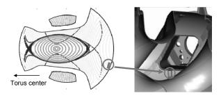
Fig. 1 Position of ion flux monitor on first-wall.
