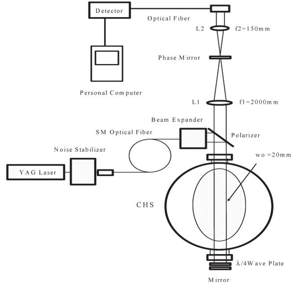
Fig. 1 Laser Imaging System for CHS.
