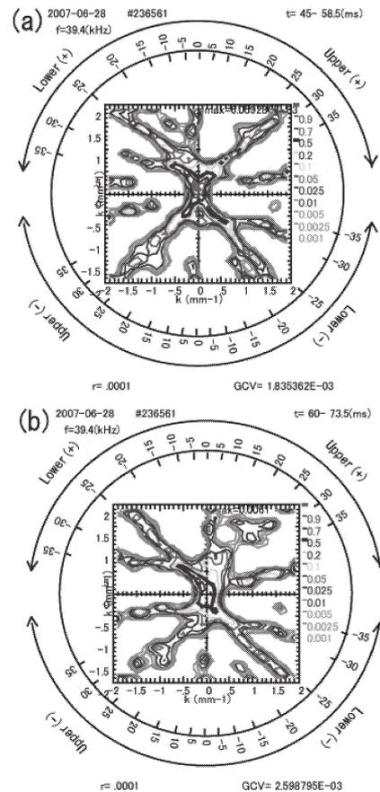
Fig. 2 Examples of the 2D distribution of the power spectra as a function of the  $k_x$  and  $k_y$ .
