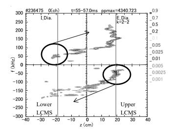
Fig.2 The spatial distribution of the measured density fluctuations before ETB transition as a function of frequency. The ETB transition happened at t=57ms.
