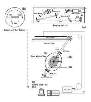
Fig.1 LPC optical System The light from the YAG laser was guided by an optical fiber, expanded in a beam expander, injected into the plasma via a port in the upper part of the CHS, reflected by a mirror, injected again into the plasma from a port in the lower part of the CHS, and then introduced into the optical detection system.
