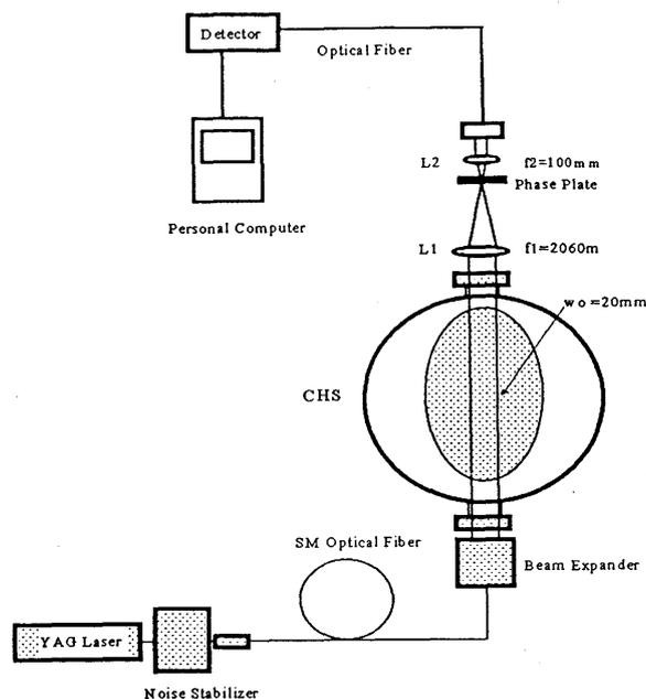
Fig.1 Laser Imaging System for CHS
