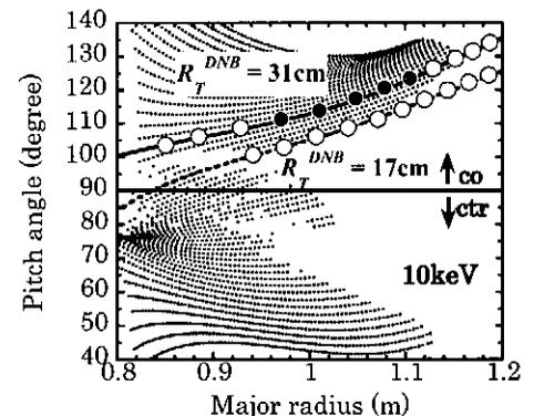
Fig. 2 Calculated confinement / loss domain for each energy component of the DNB-injected ions. The dotted area corresponds to the confinement domain. The blank area corresponds to the prompt loss domain. The solid (dashed) lines represent the beam line of DNB in  $R_T^{DNB}$  of 31 cm (17 cm). NPA observation points are plotted with circles along the beam path. Closed circles correspond to the data point where observed neutrals exceed  $3e+15$ (a.u.).
