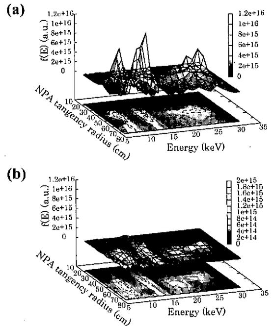
Fig. 1 Energy spectrum of neutral particles at each tangency radius of NPA for DNB injection with (a)  $R_T^{DNB}$  of 31 cm (b)  $R_T^{DNB}$  of 17 cm.
