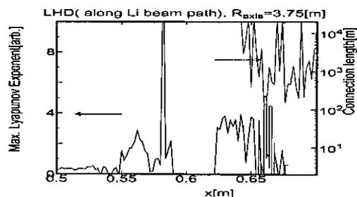
Fig. 3: The Lyapunov exponent for  $R_{ax} = 3.75$ [m] case.
