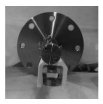
Fig. 1: Constructed calorimeter head.
