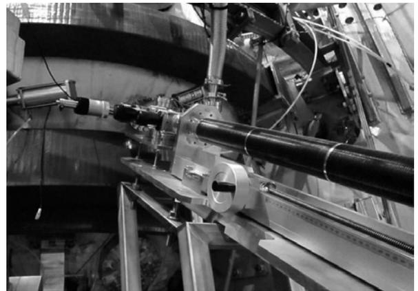
Fig. 2 Photograph of the transfer system of a sample to expose to plasmas in QUEST.
