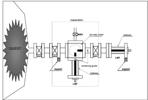
Fig. 1 Schematic diagram of a plasma exposure system equipped with the transportation of a sample.
