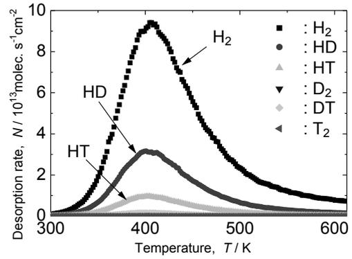
Fig. 2 Desorption spectrum, observed for SS316 exposed to glow discharge in tritium gas.
