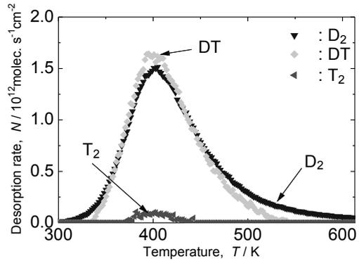
Fig. 3 Miner peaks in the desorption spectrum observed in Fig. 2.
