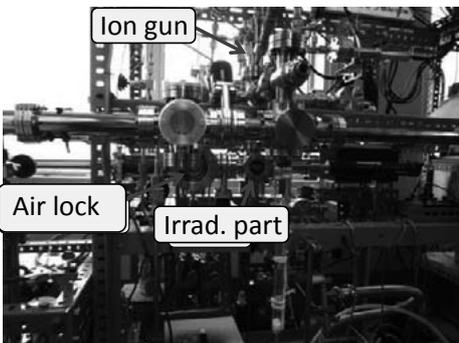
Fig. 1 New irradiation device of tritium ions.
