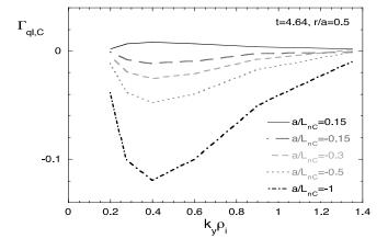
Fig.2 Wavenumber spectrum of the quasilinear carbon flux at r/a=0.5, for a range of values for the carbon density gradient parameter. Experimental parameters measured at t=4.64 sec were used in the calculations.
