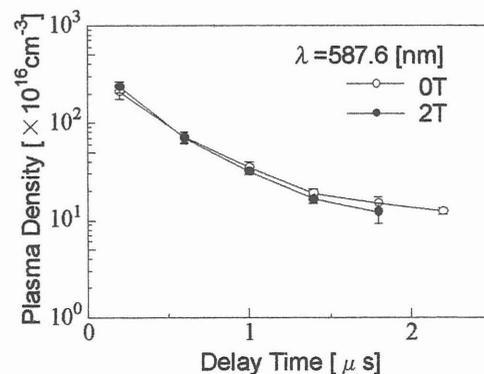
Fig.2 Difference of density decays with and without mirror magnetic field.
