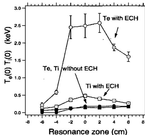
Fig. 1: Achieved central electron and ion temperatures as a function of location of the resonance zone. Open circles and squares denote the electron and ion temperature with ECH, respectively. Closed circles and squares denote the electron and ion temperature without ECH, respectively.
