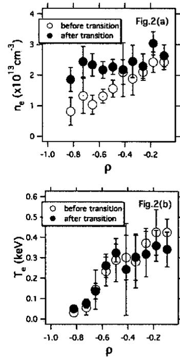
Fig. 2: Profiles of the electron density (a) and temperature (b) for ETB plasma with YAG Thomson scattering measurement.
