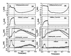
Fig. 1. Plasma current evolution in QUEST at  $B_{\rm t}{=}0.14~{\rm T}$  with the one turn cancellation coil. Left column shows  $I_{\rm CS}{=}8~{\rm kA}$  (#1932) and right one  $I_{\rm CS}{=}5~{\rm kA}$  (#1966). (a) Plasma current, (b) CS current, (c) PF26 vertical shaping coil current ( $N_{\rm PF26}{=}72~{\rm turns}$ ) and set value, (d) PF17 vertical field coil current.
