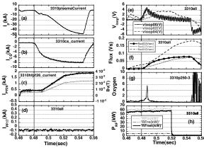
Fig. 3 The plasma current evolution for the slower OH coil current ramp-down. (a) Plasma current (b) CS current, (3) PF26 vertical shaping coil current and vertical field, (d) PF17 vertical field coil current, (e) loop voltage measured at three locations, (f) measured fluxes at three locations, (g) oxygen impurity line, and (h) 8.2 GHz RF power. (#3310)
