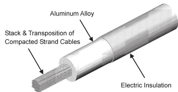
Fig. 1. Conceptual design of the indirect cooling conductor.
