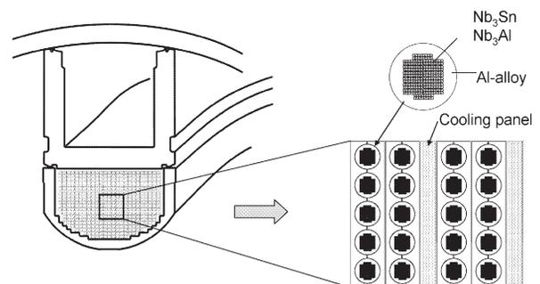
Fig. 2. Conceptual design of the indirect cooling coil.
