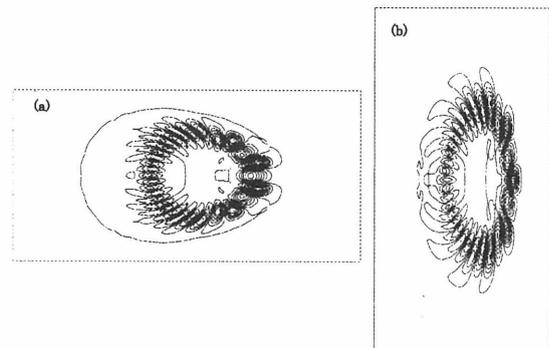
Fig.1: Contour plots of the pressure on (a) horizontally-elongated and (b) vertically-elongated poloidal sections.
