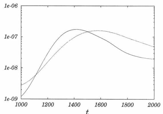
Fig.2: Energy growth caused by resistive ballooning modes. Solid and dashed lines are for runs of series A and B, respectively.
