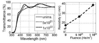
Fig. 3 Optical transmittance and electrical resistivity for GZO films irradiated with 3 keV-He<sup>+</sup>.
