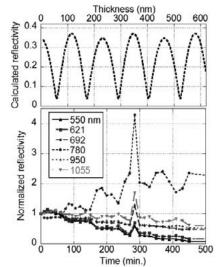
Fig. 2 Exposure time dependence of the reflectivity under H glow (bottom), and calculated dependence of the reflectivity on the deposition thickness (upper).
