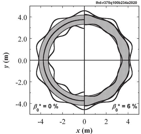
Fig. 3. Toroidal shapes of the LCFS and the plasma center on the equatorial plane calculated by the VMEC code.  $\beta_0^* = 0 \%$  and  $\beta_0^* = 6 \%$  are assumed in the left half ( $x < 0 \text{ m}$ ) and the right half ( $x > 0 \text{ m}$ ), respectively.
