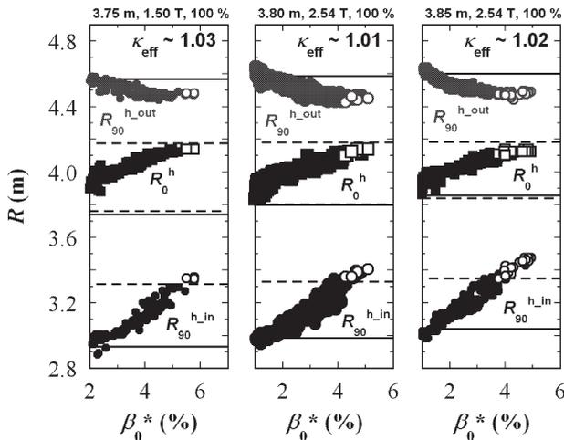
Fig. 2.  $\beta_0^*$  dependence of  $R_0^h$ ,  $R_{90}^{h,\text{in}}$ , and  $R_{90}^{h,\text{out}}$  in the outward-shifted plasmas of  $R_{\text{ax}} = 3.75 - 3.85 \text{ m}$ . Three horizontal straight (broken) lines denote  $R_1^{h,\text{out}}$ ,  $R_0^h$ , and  $R_1^{h,\text{in}}$  ( $R_1^{v,\text{out}}$ ,  $R_0^v$ , and  $R_1^{v,\text{in}}$ ) in the vacuum configuration, from top to bottom.
