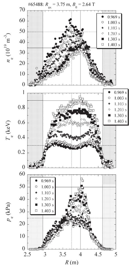
Fig. 4. Radial profiles in the highest  $n_{e0}$  discharge.
