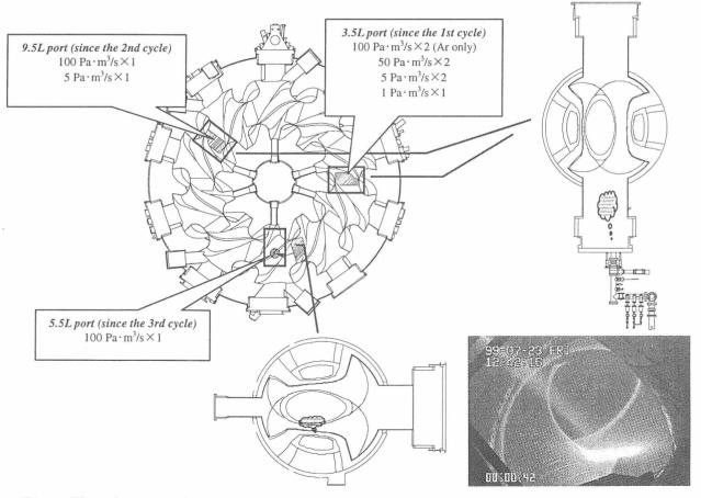
Fig. 1. The schematic of gas-puff configuration on LHD and the picture of LHD plasma with local puff.
