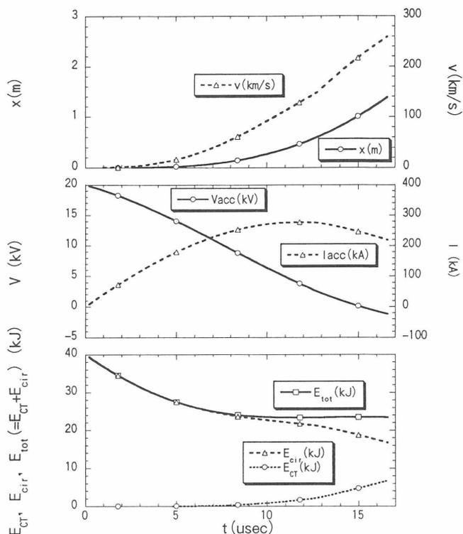
Fig. 1. Simulated waveforms of SPICA mk. I with 20 kV – 40 kJ power supply. CT mass of 0.2 mg, circuit resistivity of 20 m $\Omega$ , and external inductance of 0.48  $\mu$  H are assumed.
