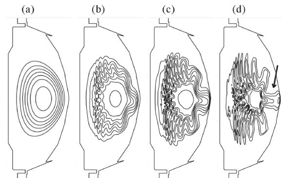
Fig.2. Time development of the poloidal pressure profile.
