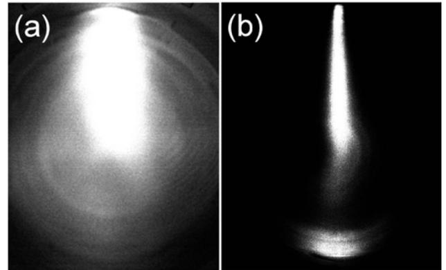
Fig. 2. Images of helium beam emission captured with CCD detector from the longitudinal direction. Helium beam is injected through (a) cone-shaped nozzle and (b) Laval nozzle.
