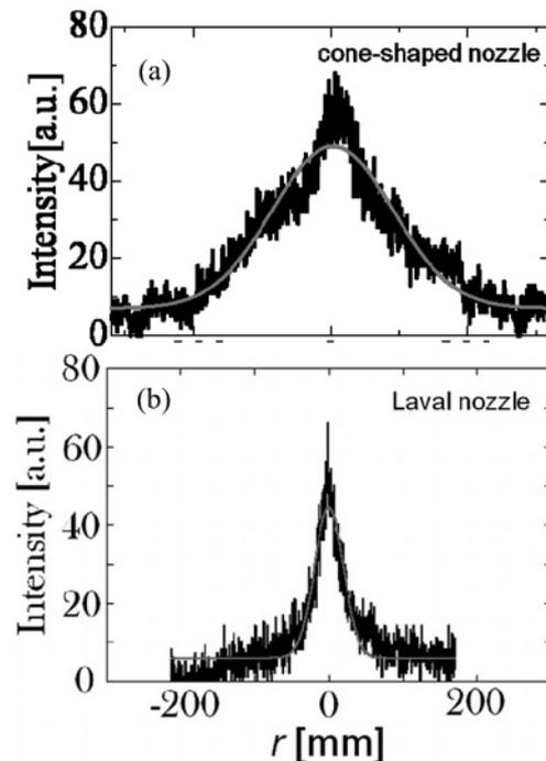
Fig. 3. Injected beam profiles with (a) cone-shaped nozzle and (b) Laval nozzle.
