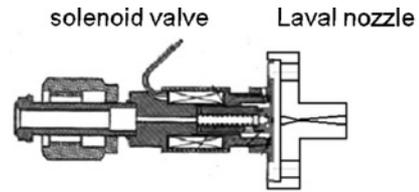
Fig. 1. Helium gas injector. Solenoid valve is directly coupled onto Laval nozzle.
