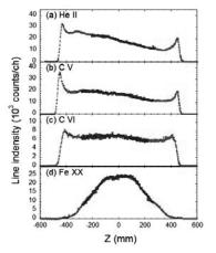
Fig.4 Vertical distributions of (a) HeII, (b) CV, (c) CVI and (d) FeXX at Y=0mm in Fig.2. Each profile is composed of three discharges traced in different colors.
