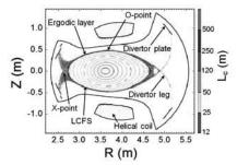
Fig.2 Magnetic field structure of LHD in  $R_{ax}$ =3.6m.
