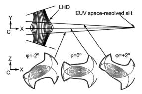
Fig.1 Poloidal cross sections at three different observation chords of space-resolved EUV spectrometer.
