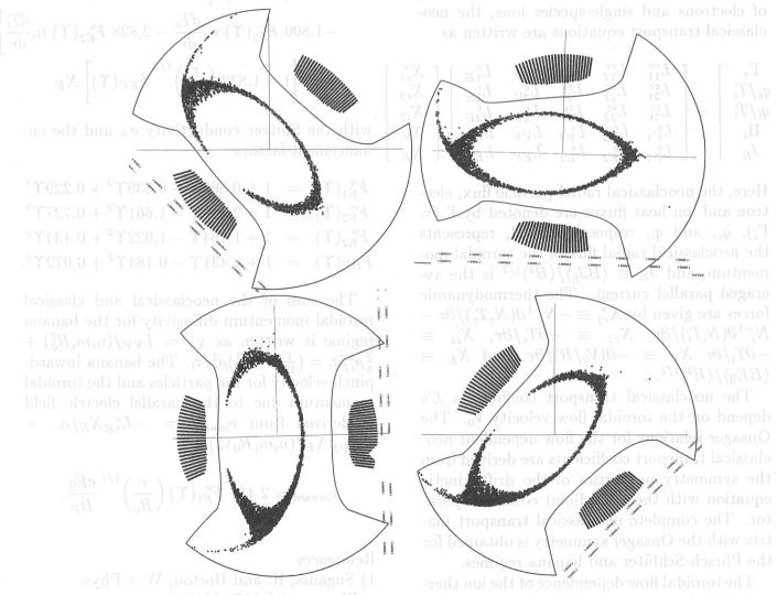
Fig.1 Poincare plot of 10KeV ions confined in chaotic field lines region.
