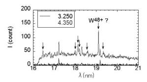
Fig. 3 EUV spectrum at wavelength region  $\sim 16-21$ nm taken by SOXMOS for #112877 at t=4.35s. Several tungsten lines are found.
