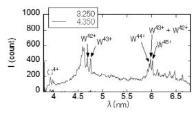
Fig.2 EUV spectrum at wavelength region  $\sim 4-6.8 nm$  taken by SOXMOS for #112877 at t=4.35s. Discrete lines of  $W^{42+} \sim W^{45+}$  ions are identified.
