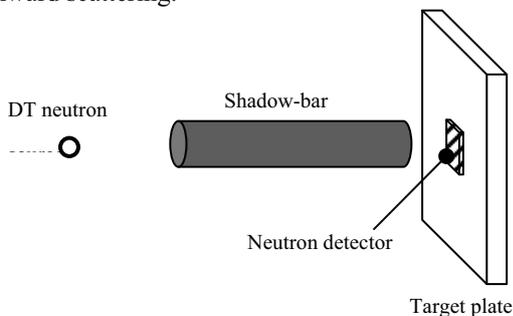
Fig. 1 Conceptual arrangement of experiment.
