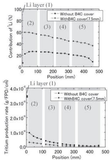
Fig. 2 Tritium production rate (upper Fig.) and contribution of  $^7\text{Li}$  ( $n,\text{no}\gamma$ ) $\text{T}$  reaction to overall tritium production (lower Fig.) as a function of the position in the Li/V test module.
