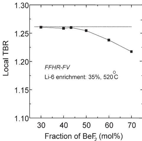
Fig.1 Local TBR as a function of the fraction of BeF<sub>2</sub> in Flibe for FFHR-FV. Blanket thickness : 60 cm, <sup>6</sup>Li enrichment : 35%, Temperature : 520 °C.
