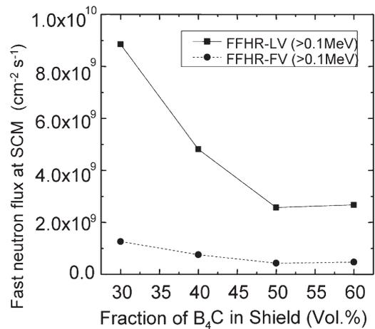
Fig.3 Fast neutron ( $E>0.1\text{MeV}$ ) flux at superconducting magnet as a function of the fraction of B<sub>4</sub>C in the shield for FFHR-LV and FFHR-FV. Blanket thickness : 54 cm for FFHR-LV and 60 cm for FFHR-FV, <sup>6</sup>Li enrichment : 35%, Temperature : 520 °C.
