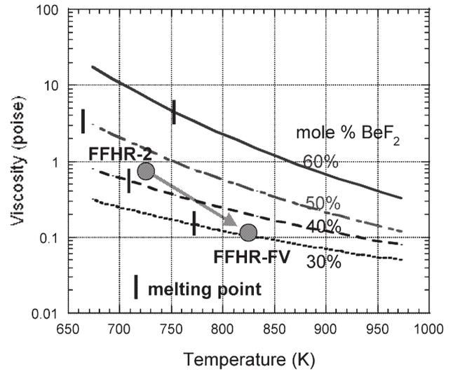
Fig.2 Viscosity of Flibe as a function of temperature and mole % of BeF<sub>2</sub>. The conditions for the minimum temperature region of the blankets of FFHR-2 and FFHR-FV are shown in the Figure.
