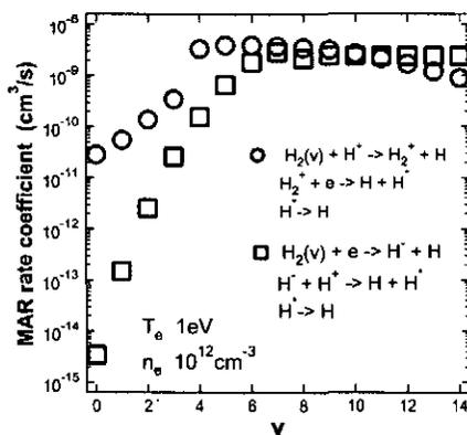
Fig.1. The MAR rate coefficients from various initial vibrational levels in  $H_2(X^1\Sigma_g^+)$ .  $T_e = 1\text{eV}$ ,  $n_e = 10^{12}\text{cm}^{-3}$ . Because the MAR rate coefficient strongly depends on initial vibrational levels of  $H_2(X^1\Sigma_g^+, v)$ , the  $v = 0-15$  levels are distinguished in our code. All atomic and molecular processes considered are listed below.
