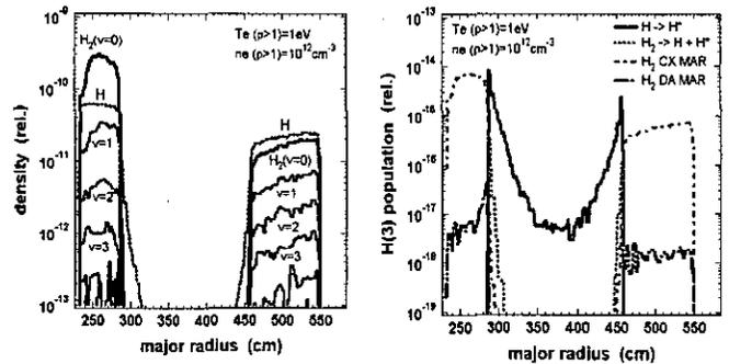
Fig.3. (a) Densities of  $H_2(X^1\Sigma_g^+, v)$  and  $H(1s)$ , and (b) Balmer  $\alpha$  emission intensities originating from various paths, along center horizontal line in Fig.2.
