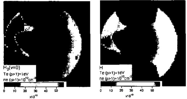
Fig.2. Density distributions of  $H_2(X^1\Sigma_g^+, v = 0)$  and  $H(1s)$ . For  $\rho \geq 1.0$  region, uniform  $T_e = 1\text{eV}$  and  $n_e = 10^{12}\text{cm}^{-3}$  are assumed.
