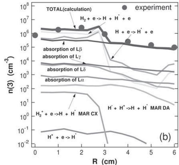
Fig.2. Population densities of excited state of atomic hydrogen with principal quantum number  $n = 3$ . As input parameter for the calculation, (a) double probe data and (b) single probe data are used, respectively.
