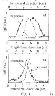
with exposure times of about 7 μs for hydrogen pellet clouds shown in Fig. 1a and 40 µs for carbon ones shown in Fig. 1b. It is seen from Fig. 1b that intensities of the carbon pellet cloud have a sharp maximum. The striking phenomenon is an appearance of "plateau" region of intensity in the hydrogen pellet cloud (Fig.1a). This "plateau" region has  $R_{pl} \approx 3-4$ mm in the transversal and  $Z_{pl} \approx 40$  mm in the longitudinal directon. It is supposed that this re-
