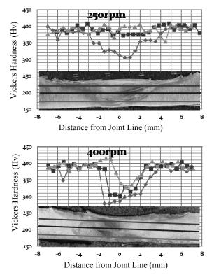
Fig. 1 Cross-sectional Vickers hardness distributions in F82H/ODS joints joined by FSW.
