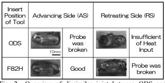
Fig. 2 Overview of dissimilar joint between ODS and F82H by FSW.
