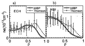
Fig.2 Obtained density profiles from HIBP. For comparison, the profile measured with Thomson scattering is shown. a) ECH and b) NBI plasma.
