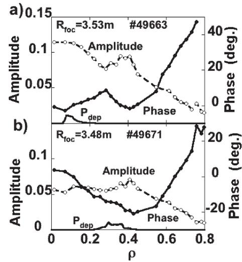
Fig. 3: FFT amplitude and phase profiles are plotted for the antenna focal point settings of a)  $R_{foc}=3.53\text{m}$  and b)  $R_{foc}=3.48\text{m}$  with calculated absorption power profiles
