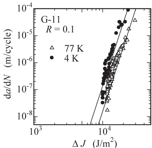
Fig. 1. Fatigue crack growth rate in G-11 woven laminates at 77 K and 4 K (load ratio  $R = 0.1$ , frequency 3 Hz)
