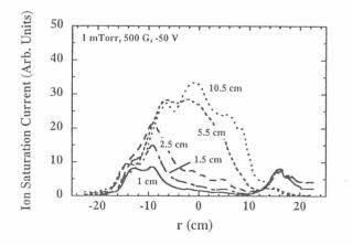
Fig. 2. Radial profiles of ion saturation current  $I_{is}$ , changing a distance from the plate (1 mTorr, 500G, - 50V)
