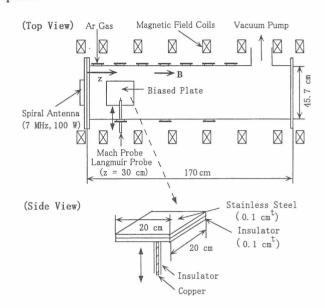
Fig. 1. Schematic view of experimental setup
